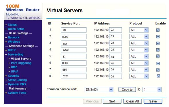
Figure 8-1 Port Mapping on Router
